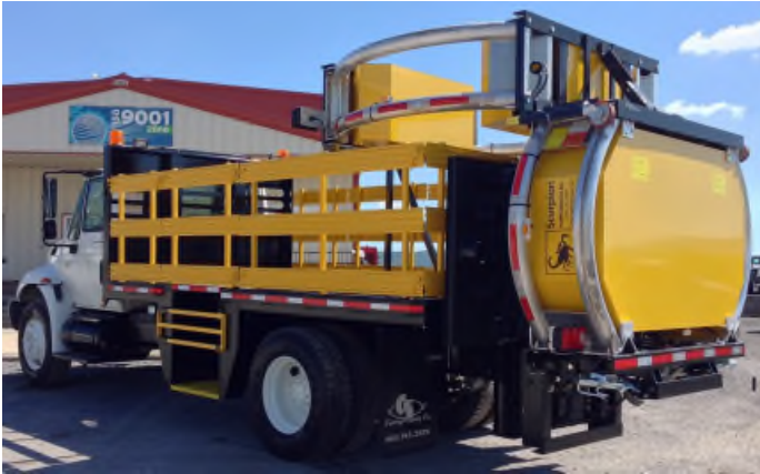
TRUCK WITH ATTENUATOR STOWED
