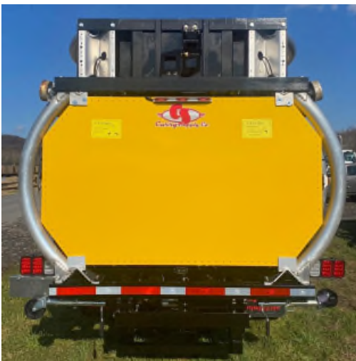
REAR VIEW WITH ATTENUATOR STOWED
